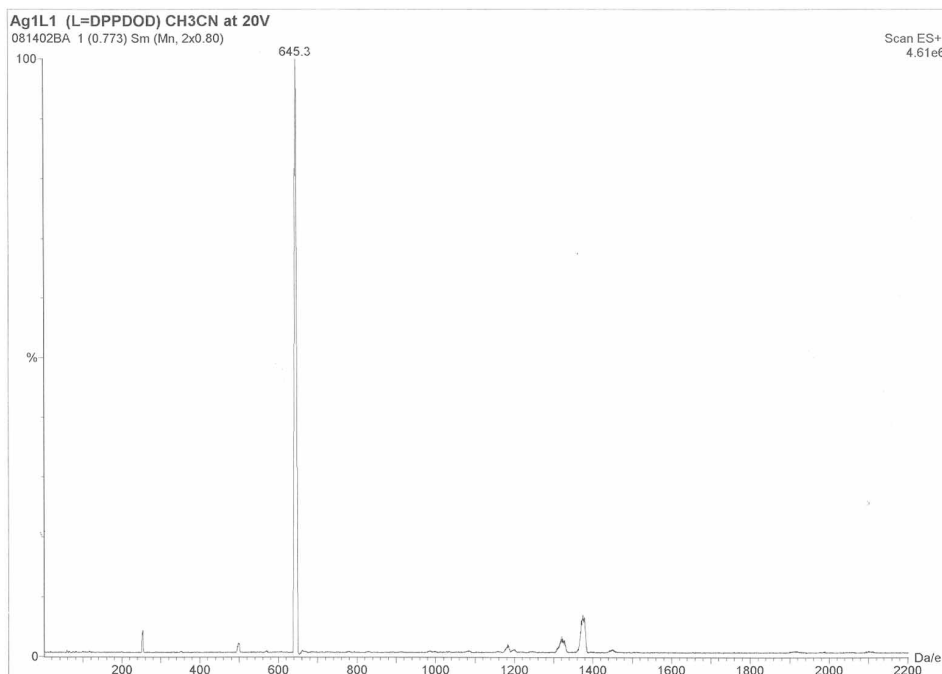
Figure 4. Electrospray mass spectrum of DPPDOD:AgBF 4 ( C_L/C_M = 1.0 ) at a cone voltage of 20 V.
